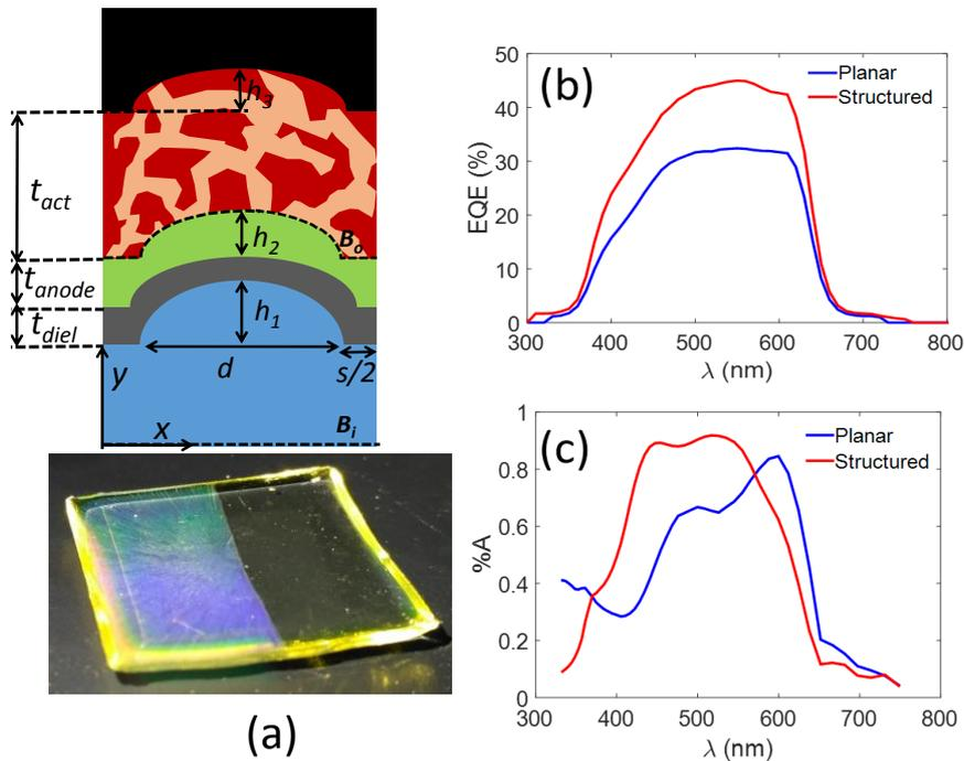
**Fig. 1** (a) Schematic device architecture employed (above) and structured substrate (below), (b) External quantum efficiency of planar and structured devices, (c) Computed absorptances of planar and structured devices.
